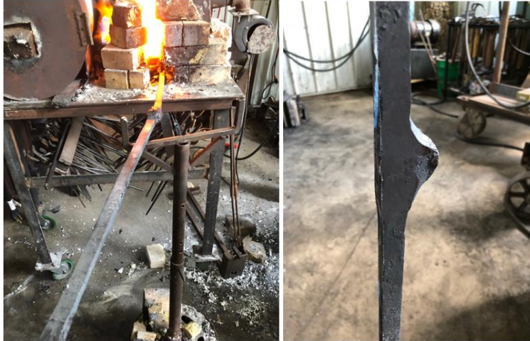
Figure 6 forging the steel for the cutting edge
