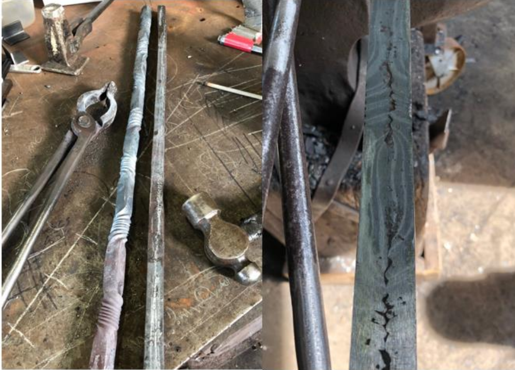
Figure 5, forging the alternating twists
