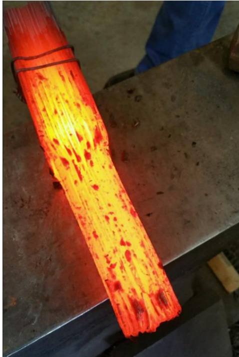
Figure 5 forge welding the billet
