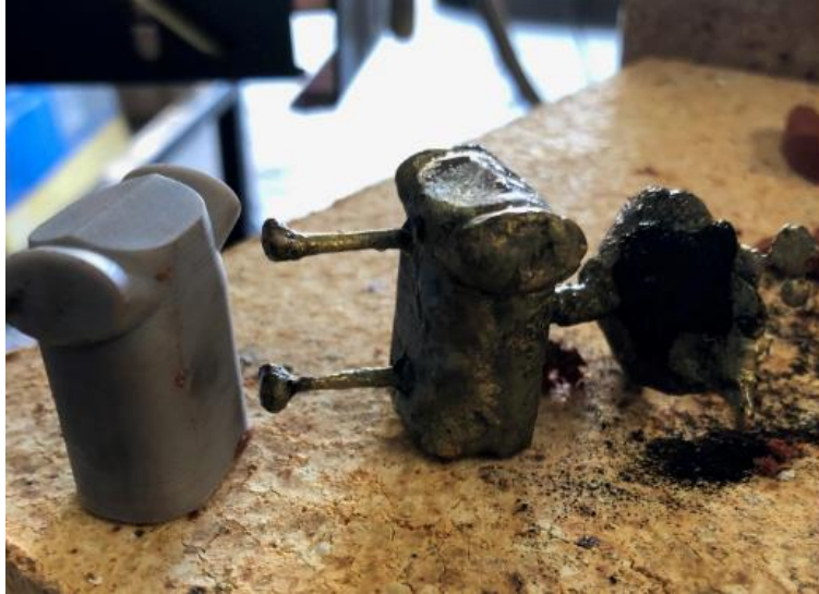
Figure 11 the pommel removed from the mold
