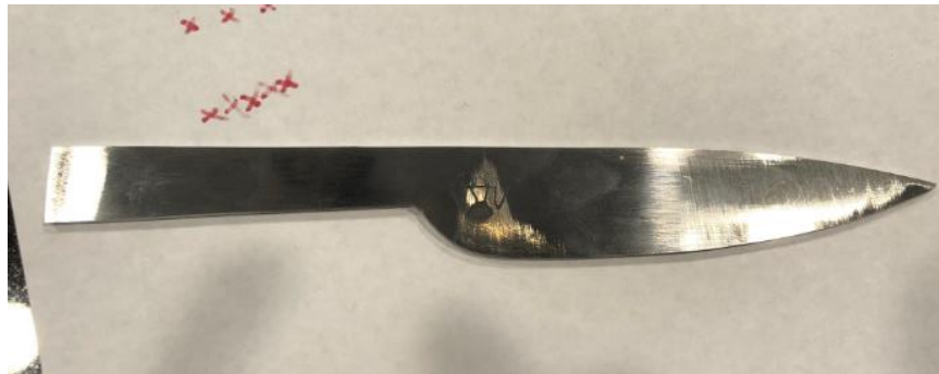
Figure 7 the forged blade following rough grind
