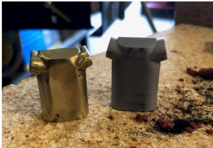
Figure 12 the cast pommel following rough clean-up
