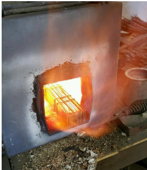
Figure 4 heating up the stacked billet
