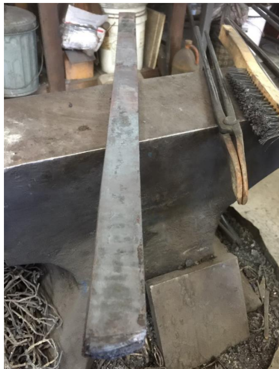
Figure 6 the completed billet
