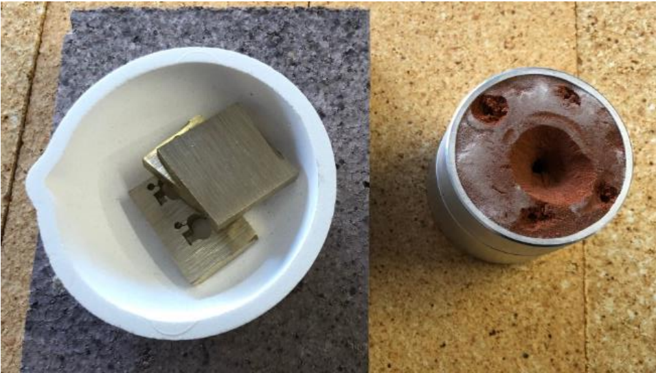
Figure 10 assembled mold and brass in crucible
