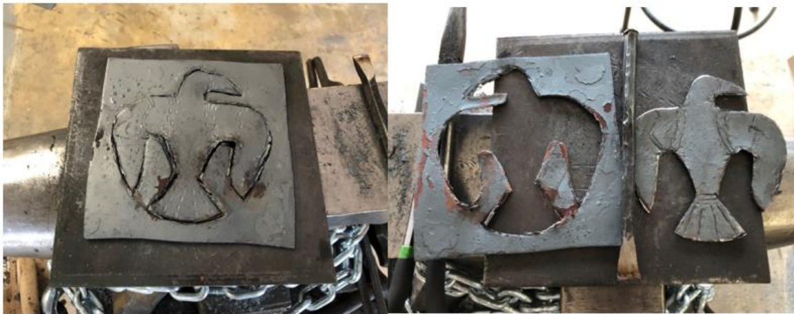
Figure 21 chiseling out the lock plates
