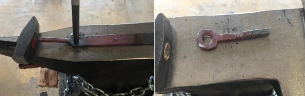
Figure 20 drifting the hole in the lock hasp
